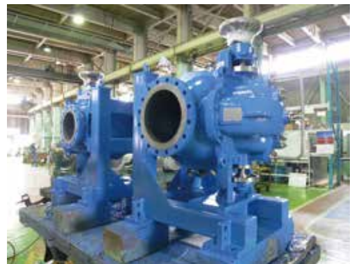
Potable Water Pump CDMV350×300mm, 1,137m 3 /h, 45m, 185kW
