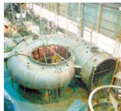
Fabricating volute casing of 3,000mm size drainage pump, Japan
