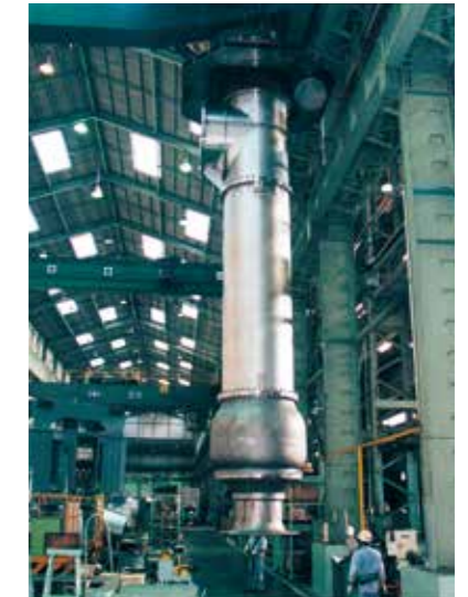
Cooling water pump for P.A.I. Shuaiba, Kuwait (Size:1,400mm, Driver:1,500kW)
