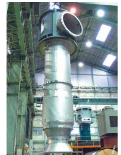
Circulating water pump for Meseieed A IWPP project, Qatar (Size:1,500mm, Driver:1650kW)
