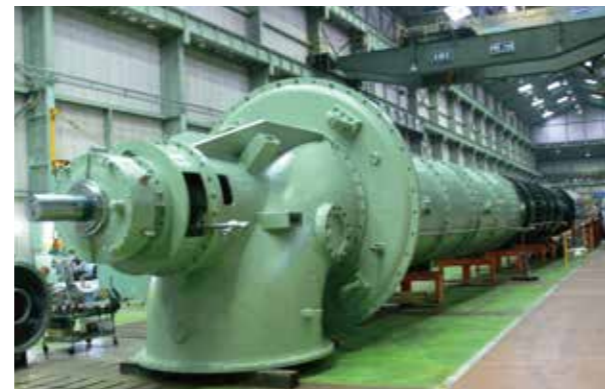
Rain water drainage pump, Jaan (Size: 2,000mm, Driver:3,100kW)
