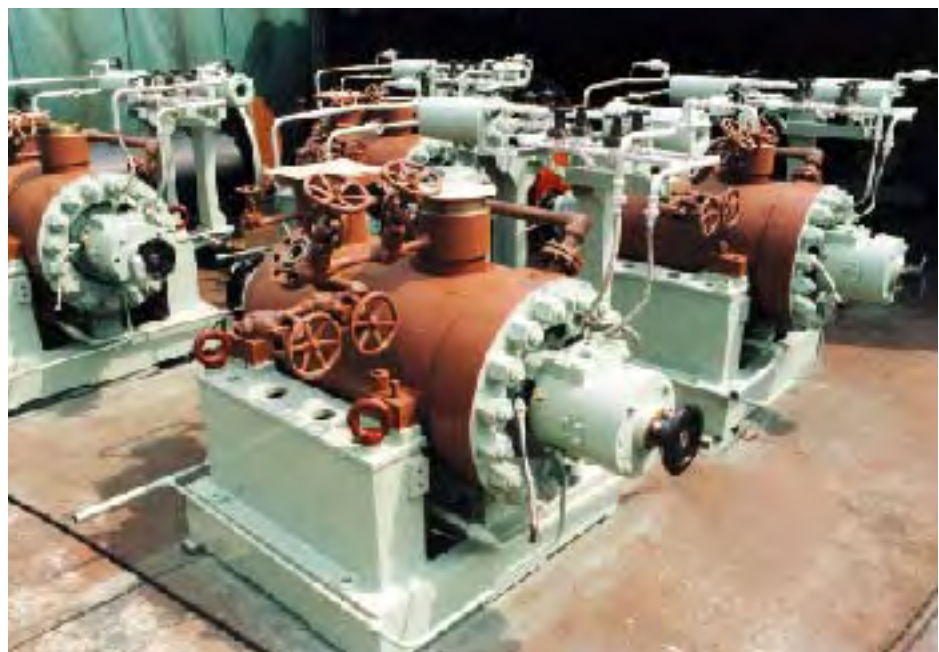
Barrel casing boiler feed pump 3,130psi-3,030U.S.gpm-6,150min -1 -6,500HP Dalian No.4 Power Plant(China) , 350MW×2units
