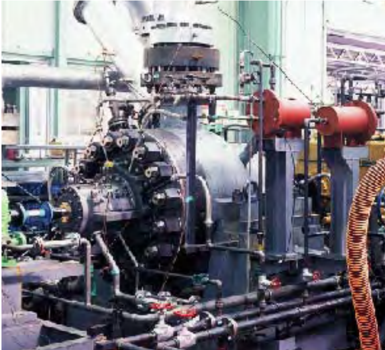
Barrel casing boiler feed pump(100% B.F.P.) 9,110ft-6,230 U.S.gpm-5,330min -1 -16,890HP
