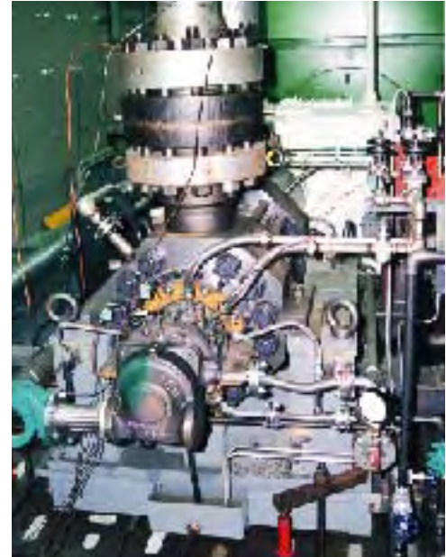
Segmental ring-section casing boiler feed pump 9,310ft-3,114 U.S.gpm-5,840min -1 -9,650HP
